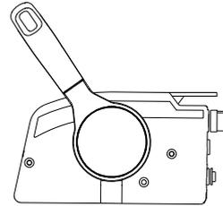
2. Pull up the neutral interlock rigger and move the remote control lever quickly and firmly from neutral to reverse.
