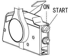
7. Immediately after the engine starts, release the main switch and allow it to return to “**ON**”(on).
