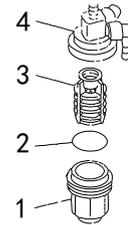
1. filter cup 2. O-ring 3. filter element 4. filter housing
